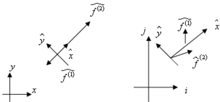
For the bar element, force and displacement are only assumed on the axial direction
