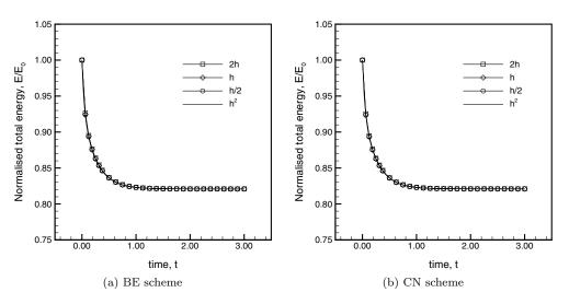
FIG. 1. Normalized total energy  $E/E_0$  dissipation profiles from time t = 0 to t = 3.0 with a fixed mesh size of h = 1/128 and different time-step sizes  $\Delta t = 2h, h, h/2, h^2$ .
