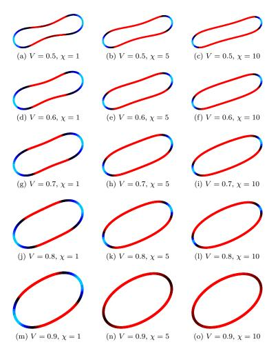
FIG. 4. The equilibrium vesicle shapes of V = 0.5, 0.6, 0.7, 0.8, 0.9 under shear flows of  $\chi = 1$ , 5, 10. The elastic tension distributions are represented by 20 contour levels. The contour levels are scaled individually with 10 levels in the positive value (red end) representing tension and 10 levels in the negative value (blue end) representing compression, while the inflection point is represented by the black end.
