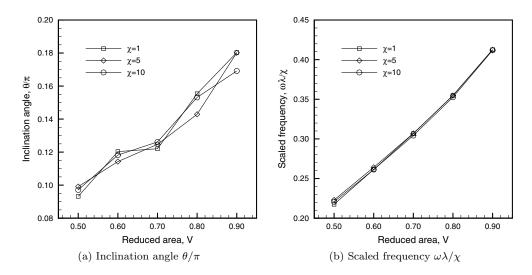
FIG. 5. Inclination angle  $\theta/\pi$  and scaled tank-treading evolution frequency  $\omega\lambda/\chi$  of the vesicle in terms of reduced area V at their equilibrium shape under dimensionless shear rate  $\chi = 1, 5, 10$ .
