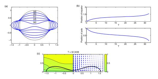
Figure 8: Transient dynamics for the oblate drop in Fig. 6 with (Q, R) = (2, 10) and  $Ca_E = 0.315$ . Panel (a): The dashed curve represents the initially spherical drop shape. Time T = 1.4, 4.7, 18.7, 30, and 32.3 for curve (a), (b), (c), (d), and (e), respectively. Panel (b): Position of the equator (top) and pole (bottom) versus time. Panel (c): Contour plots of the electric potential (left) and circulation plots (right).
