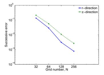
Figure 4: Successive errors for the electric interfacial force ( $F_E$ ) in r (solid curve) and z-direction (dashed curve), as a function of the grid number N. The rate of convergence is nearly second order.
