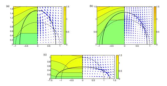
Figure 7: Steady state contour plots of the electric potential (left) and circulation plots (right) for (a) the prolate A drop with (Q, R) = (0.1, 0.1) and  $Ca_E = 0.325$ , (b) the prolate B drop with (Q, R) = (50, 0.04) and  $Ca_E = 0.305$ , and (c) the oblate drop with (Q, R) = (2, 10) and  $Ca_E = 0.304$ . The dashed curve represents the initially spherical drop shape.
