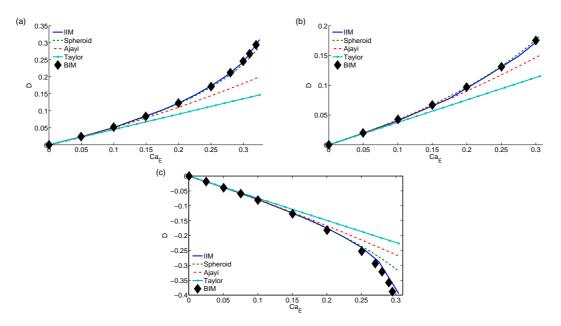
Figure 6: Equilibrium drop deformation versus  $Ca_E$  from our IIM (solid), spheroidal model (dashed), Ajayi's second-order approximation (dotted-dashed), Taylor's results (dotted-solid) and the BIM (symbol). (a) Prolate A drop with (Q,R) = (0.1,0.1). (b) Prolate B drop with (Q,R) = (50,0.04). (c) Oblate drop with (Q,R) = (2,10).
