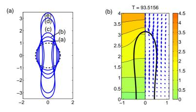
Figure 9: Transient dynamics for the prolate A drop in Fig. 6 with (Q, R) = (0.1, 0.1) and  $Ca_E = 0.37$ . Panel (a): The dashed curve represents the initially spherical drop shape. Time T = 3, 20.3, 50.8, 77.2, and 93.4 for curve (a), (b), (c), (d), and (e), respectively. Panel (b): Contour plots of the electric potential (left) and circulation plots (right).
