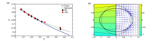
Figure 5: (a) Comparison of the steady state deformation (D) versus conductivity ratio R between Taylor's approximation (Eq. (4.3), solid), the spheroidal model (dashed), the IIM, and VOF results [41]. Other parameters are: Q=10,  $\mu_r=1$ , and  $Ca_E=0.18$ . (b) Steady state contour plots of the electric potential (left) and circulation plots (right) with (Q,R)=(10,1/1.81) and  $Ca_E=0.18$ . The dashed curve represents the initially spherical drop shape.
