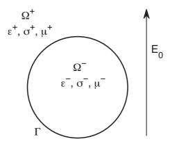
Figure 1: Sketch of the problem: A leaky dielectric viscous drop (in domain  $\Omega^-$ ) immersed in another dielectric fluid (in domain  $\Omega^+$ ), with an external electric field  $E_0$  in the z direction. Subscript '+' and '-' denote the exterior and interior fluids, respectively.
